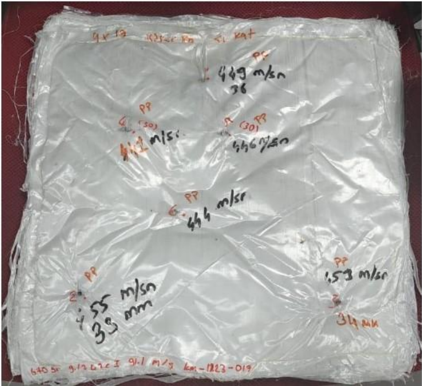
Ballistic package weight: 4.080 g/m² (51 layers/80 g/m²) (NIJ 0101.04)
