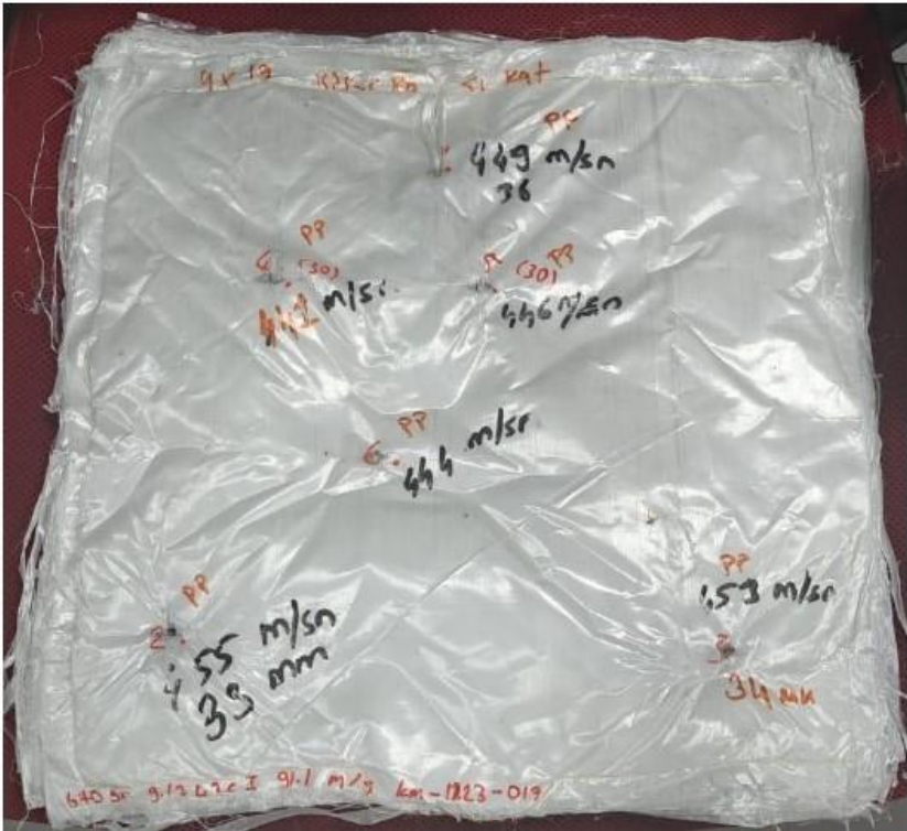
Ballistic package weight: 4.080 g/m 2 (51 layers/80 g/m 2 ) (NIJ 0101.04)
